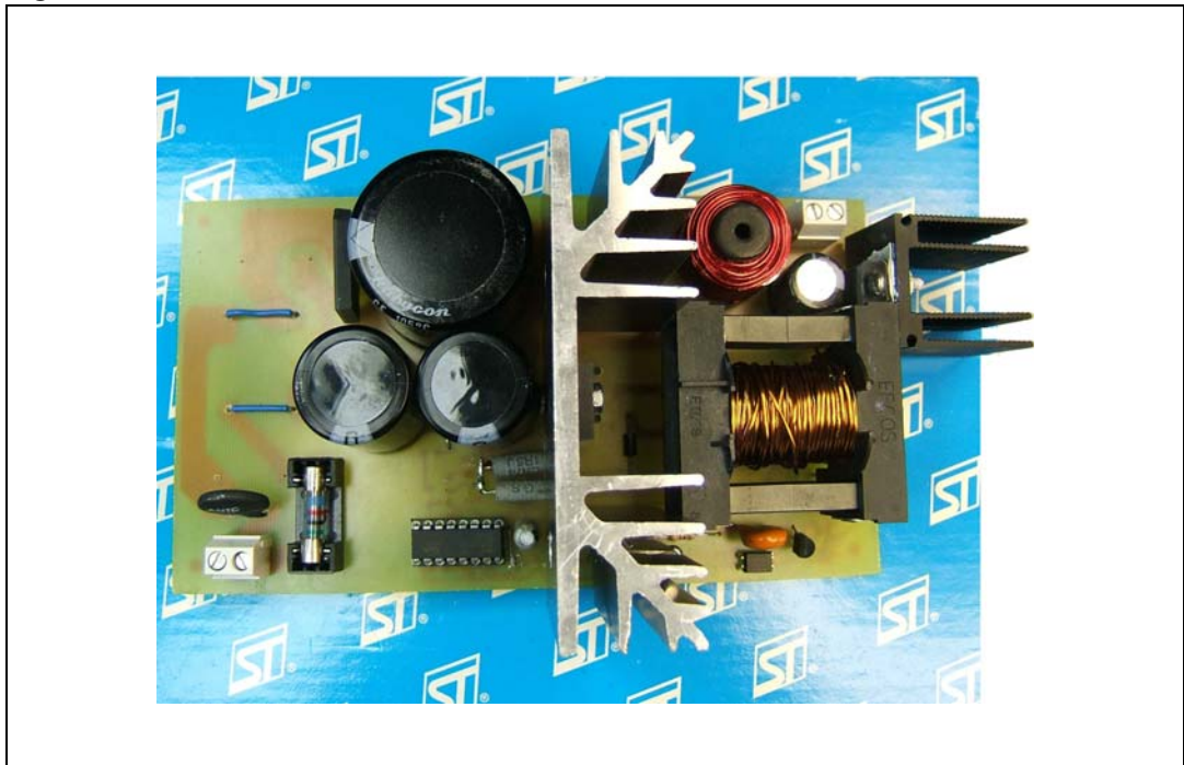
Figure 1. 160 W off-line forward converter, evaluation board
