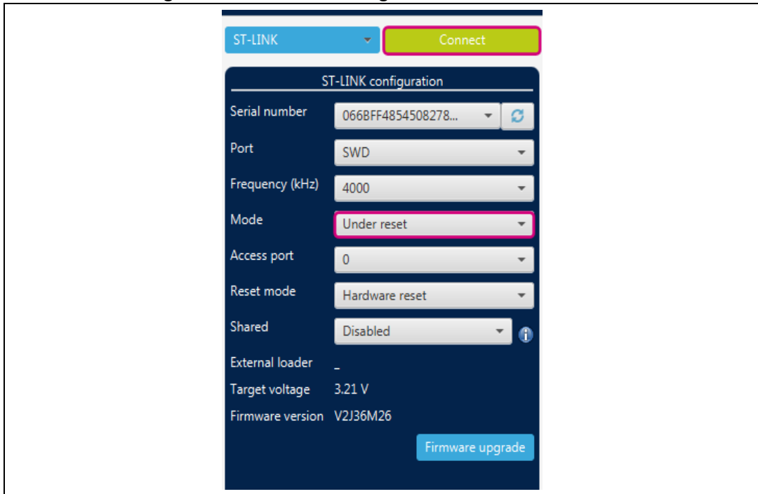
Figure 19. STM32CubeProgrammer connection menu
